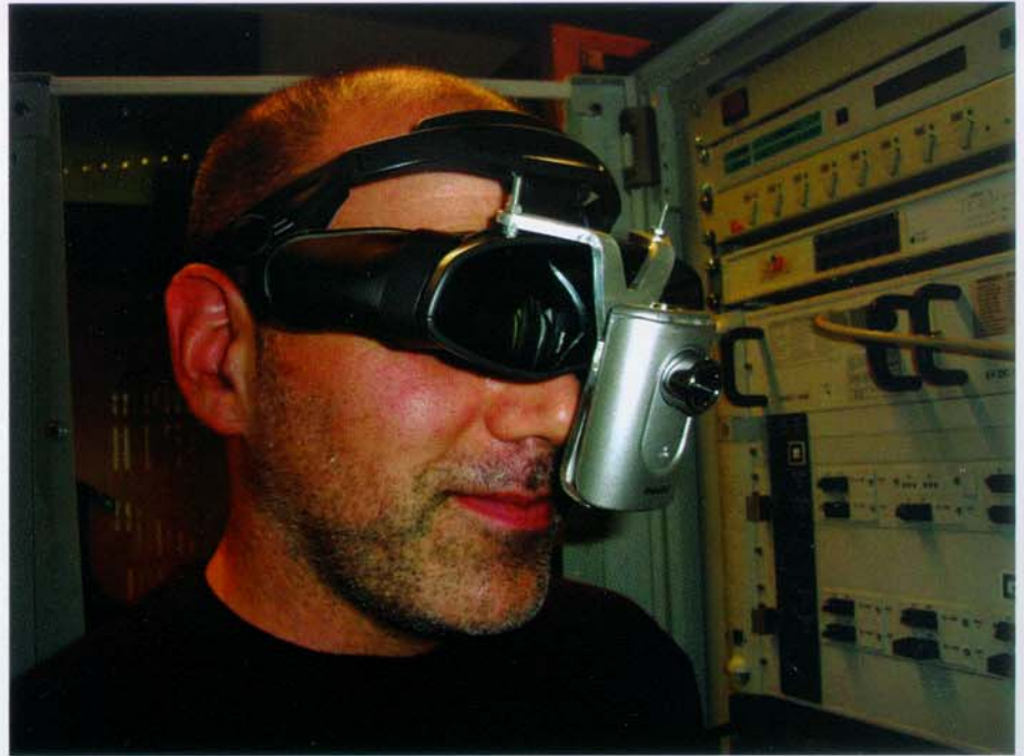
The head-mounted display brings the real and the virtual world together.
